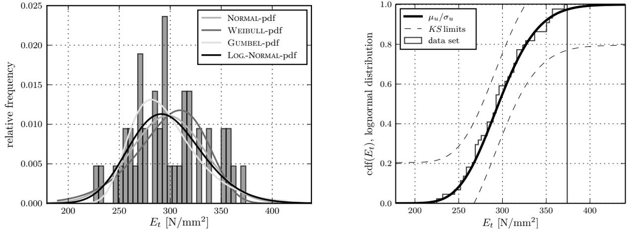
(a) Probability density functions and histogram of  $\underline{E}_t$ (b) LOG-NORMAL cumulative distribution function for  $E_t$  and empirical cumulative distribution of  $\underline{E}_t$ , limits for KS statistic Eq. (27)Figure 4. All admissible distributions for  $E_t$  and the best fitting distribution within KS limits for  $\alpha = 0.05$ .
