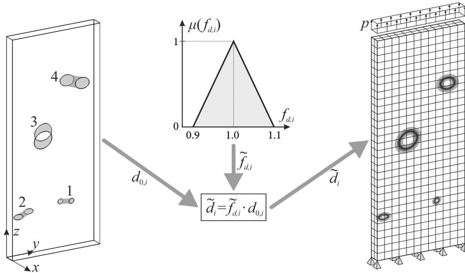
Figure 7. Original geometrical model and FE model with fuzzy sized knots due to fuzzy knot diameter  $\tilde{d}_i$ .
