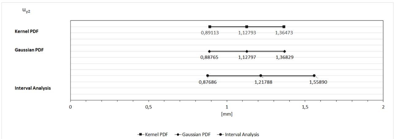
Figure 7.  $u_{y2}$ : interval analysis bounds and *Kernel* and *Gaussian PDF*  $\mu_u \pm 3\sigma_u$ .
