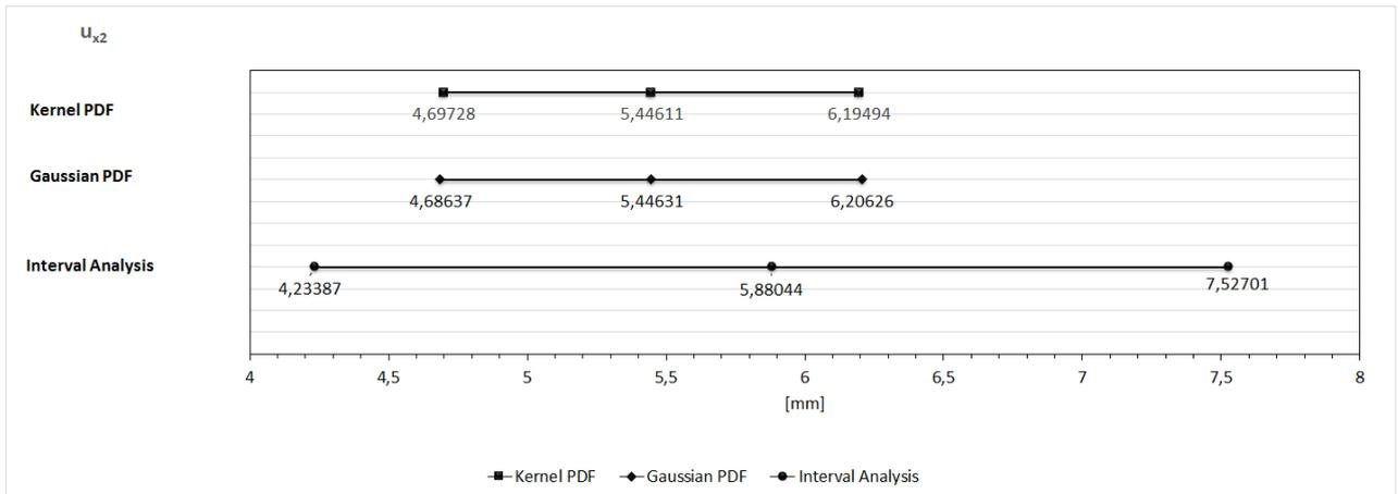
Figure 6.  $u_{x2}$ : interval analysis bounds and *Kernel* and *Gaussian PDF*  $\mu_u \pm 3\sigma_u$ .
