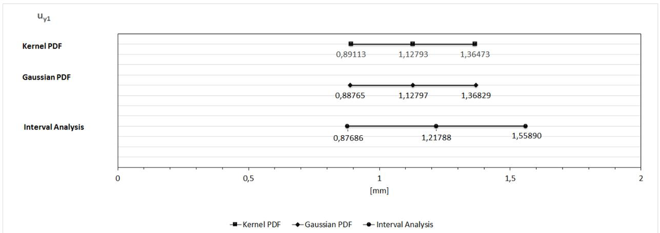
Figure 5.  $u_{y1}$ : interval analysis bounds and Kernel and Gaussian PDF  $\mu_u \pm 3\sigma_u$ .
