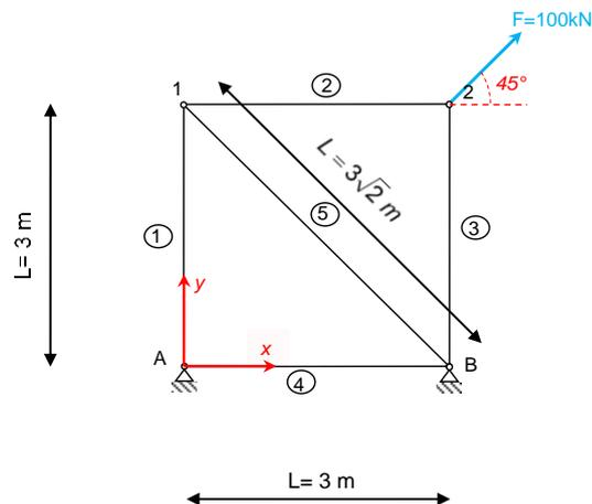
Figure 1. Sketch of benchmark truss system.
