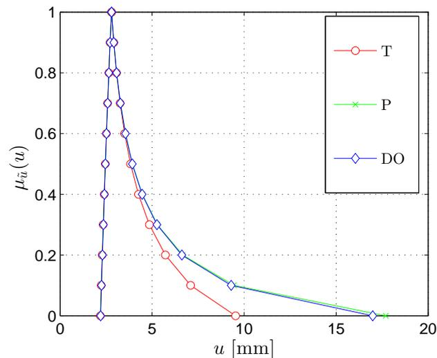
Figure 5. Membership function of amplitude of steady-state vertical displacement.
