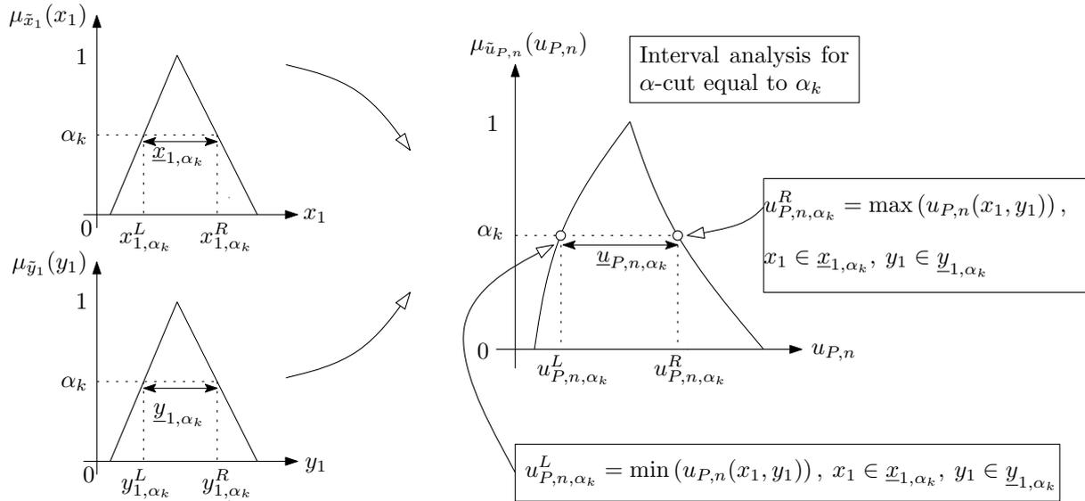
Figure 1. Schematic Representation of Fuzzy Analysis Applying  $\alpha$ -level Optimization.
