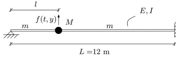
Figure 3. Steel beam subject to point load.
