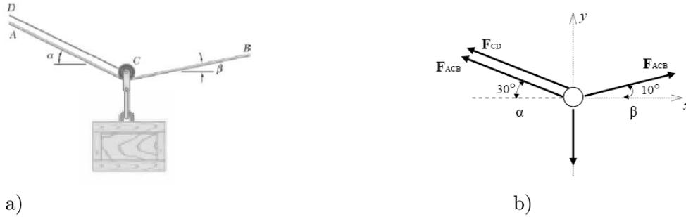
Figure 2. a) A crate suspended from a pulley can roll freely on the support cable ACB and is pulled at a constant speed by cable CD; b) Free-body diagram.
