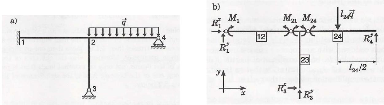
Figure 3. Planar frame (a) and its fundamental system of internal parameters (b), after (Kulpa et al., 1998).
