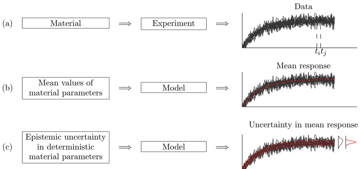
Figure 1. Scheme of an experiment and different approaches to parameter identification.
