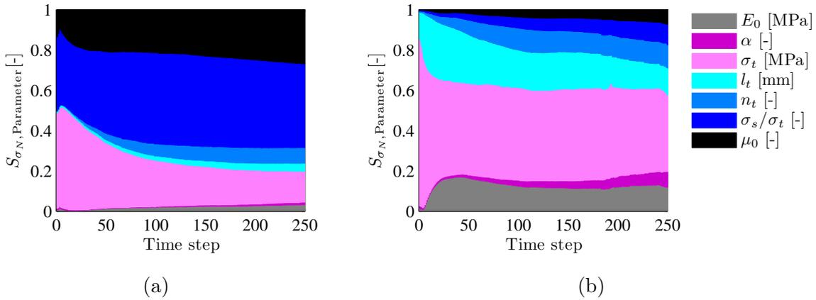
Figure 6. Sensitivity analysis for uniaxial compression test (a) and three-point-bending test (b) based on Sobol indices computed from PCE approximation.
