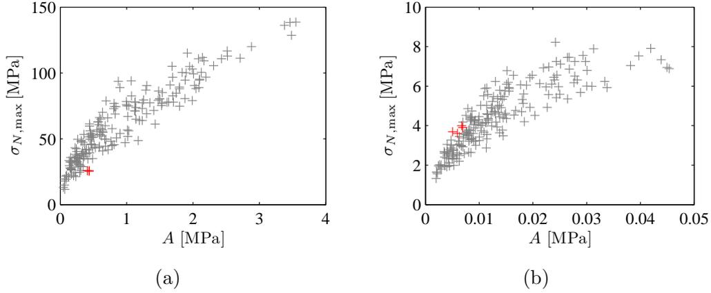
Figure 5. Comparison of integrals of training and experimental curves for uniaxial compression test (a) and three-point-bending test (b).
