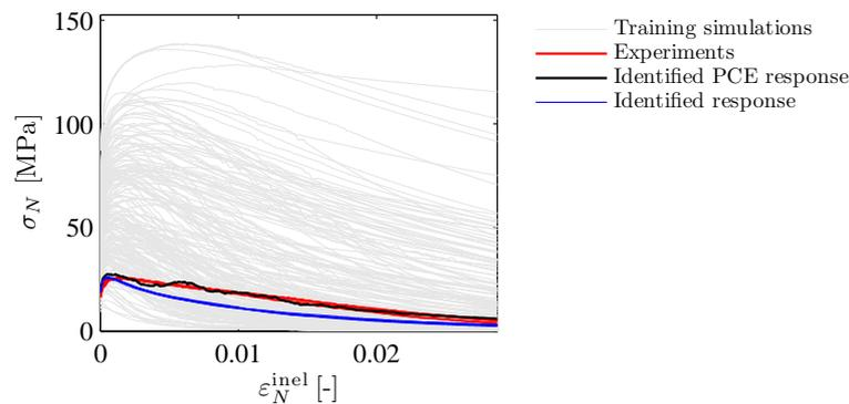
Figure 3. Comparison of experimental data and model response corresponding to the identified parameters for the uniaxial compression test.
