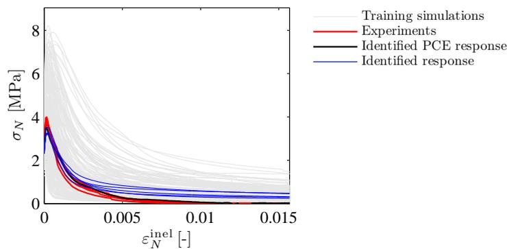
Figure 4. Comparison of experimental data and model response corresponding to the identified parameters for the notched three-point-bending test.
