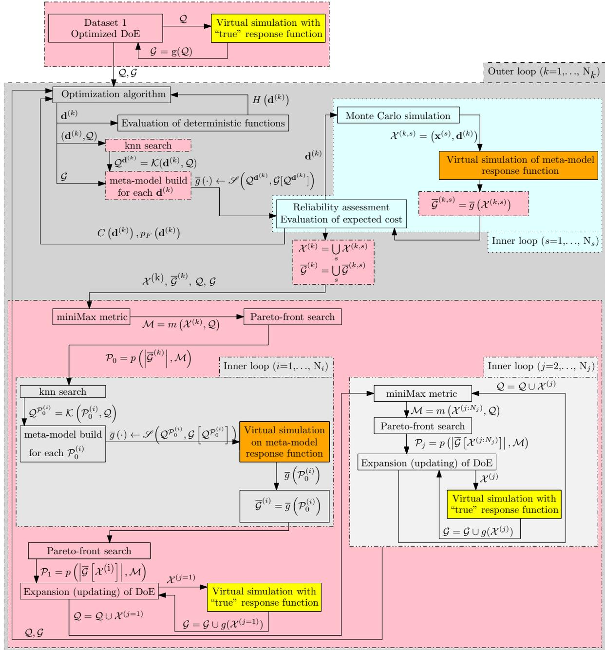
Figure 1. Schematic representation of a double-loop RBDO problem extended to the meta-model update.
