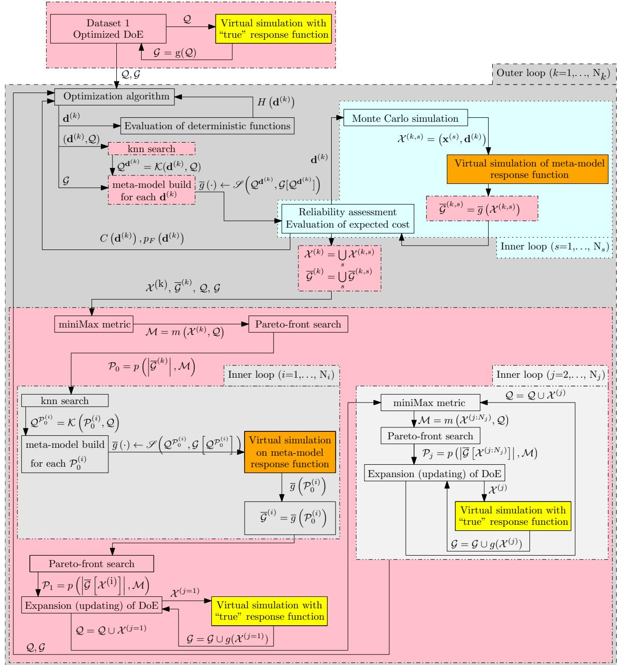
Figure 1. Schematic representation of a double-loop RBDO problem extended to the meta-model update.
