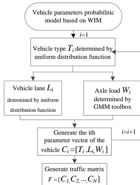
Figure 1. A framework for stochastic traffic flow simulation based on the Monte-Carlo approach (In this article, GMM refers to Gaussian mixture model).
