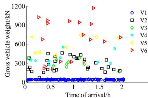
Figure 3. A stochastic fatigue traffic flow sample.
