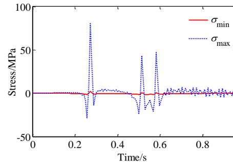
Figure 6. Stress-time curves of roof U-rib of the steel box girder.
