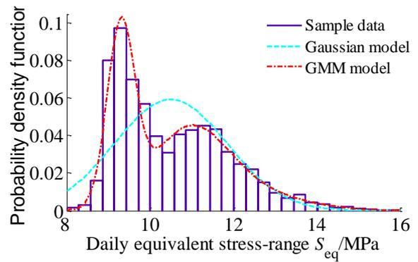
Figure 8. Fatigue stress probability density of the rib-to-deck detail of driveway under the random traffic flow samples.
