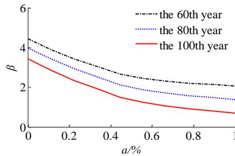
Figure 10. Influence of increase of vehicle weight on fatigue reliability index.
