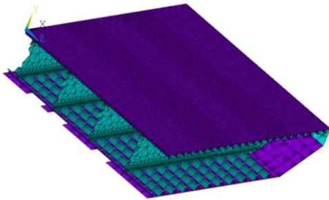
Figure 5. Finite element model of a steel box girder.
