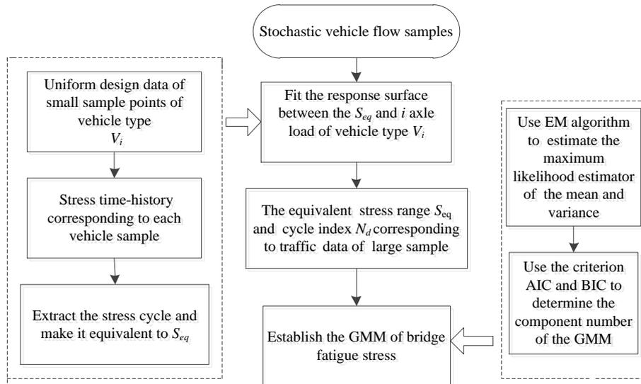
Figure 4. Probability analysis process of fatigue stress.
