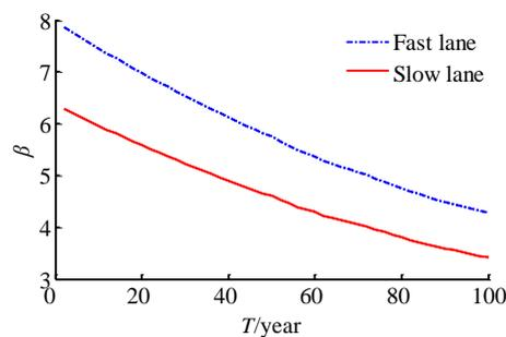
Figure 9. Fatigue reliability index of the rib-to-deck detail during the operation period.
