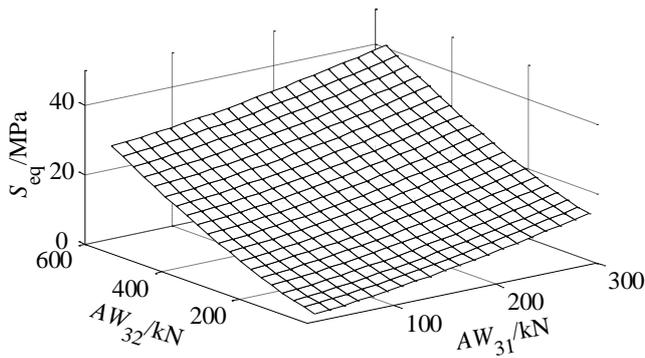
Figure 7. Response surface of  $S_{eq}$  and axle weight of V3.
